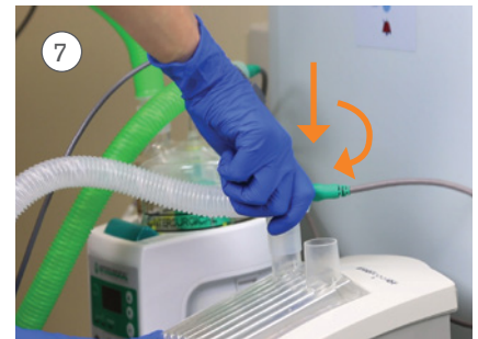
Connect the expiratory heated wire limb to the 22mm male connector of the InterCooler cassette
