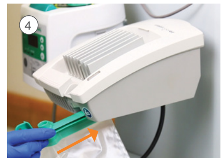
Insert the fluid collection bag into the InterCooler
