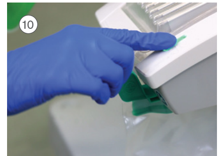
Turn on the InterCooler by pressing the power button . The button will illuminate green if the system is set up and functioning correctly
